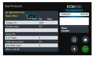
Plate Handler Tap for HT-100 or HT-200 HT Plate Handler settings.
