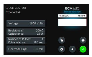
Voltage, Resistance, Capacitance, Number of pulses, Pulse Interval, and electrode gap may be modified by tapping on the gray icons for each. Green Accept icon may be tapped to proceed to Run Protocol screen.
