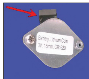
Remove Battery Insulating Tab.
